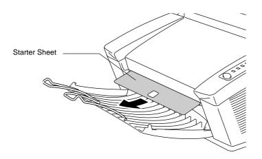
Fig. 5-16 Ejecting the Starter Sheet
