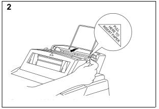
Open the cover of the multi-purpose sheet feeder 2.
