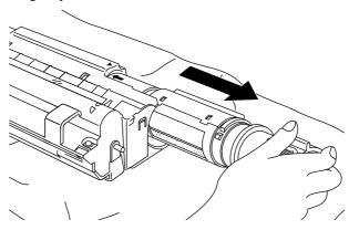
Fig. 5-5 Removing the Old Toner Cartridge
