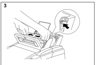
Pushing and sliding the tabs, move the paper guides horizontally to the widest position.
