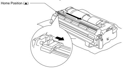
Fig. 5-23 Cleaning the Primary Corona Wire
