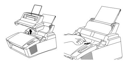
Fig. 6-4 Paper Jam under Feeder 1
