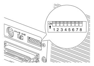
Fig. 4-2 Setting the Serial Interface Parameters
