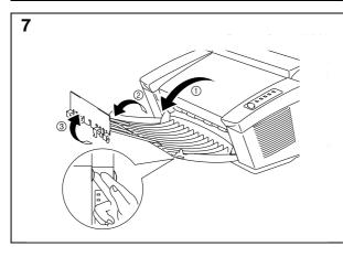
Open the output tray. ( 1 ) Extend the extension support wire ( 2 ) and set the paper stopper ( 3 ).
