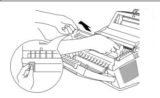
Fig. 5-2 Removing the Drum Unit
