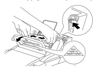
Fig.2-4 Opening the Feeder and Moving the Paper Guides
