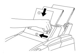
Fig. 2-9 Moving the Paper Guide
