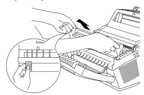
Fig. 5-10 Removing the Drum Unit
