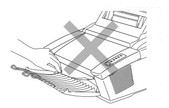
Fig. 6-7 Do Not Pull the Jammed Paper from the Output Tray
