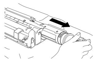
Fig. 5-12 Removing the Toner Cartridge
