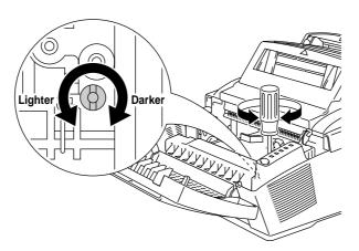
Fig. 5-17 Adjusting the Print Density Dial
