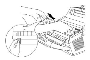
Fig. 5-15 Installing the Drum Unit
