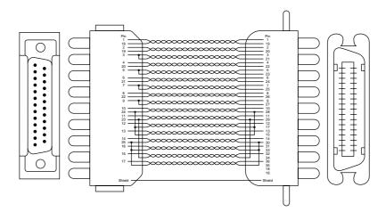
Fig. A-1 Parallel Interface Cable
