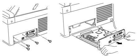
Fig. 4-4 Remove the main controller board
