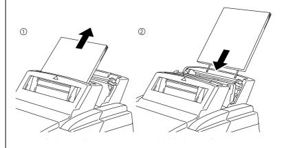
Fig. 2-7 Loading Paper in Feeder 2
