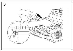
Holding the drum by its handles, install it into the printer. The drum will slide easily into place.
