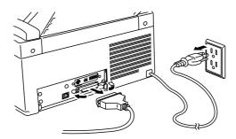
Fig. 4-3 Unplug the power cord and disconnect the interface cable
