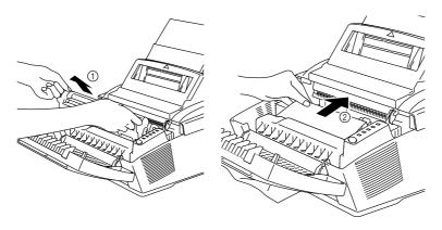
Fig. 6-6 Paper Jam Inside the Printer
