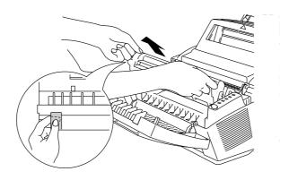
Fig. 5-26 Removing the Drum Unit Assembly
