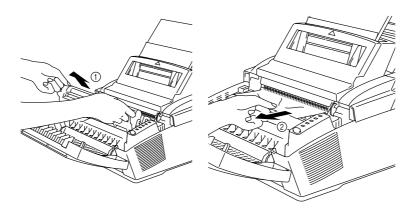
Fig. 6-5 Paper Jam near the Drum Unit
