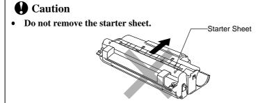
Fig. 5-14 Do Not Remove the Starter Sheet
