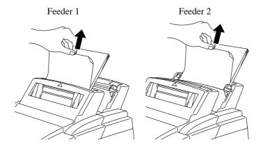
Fig. 6-3 Paper Jam in the Feeders
