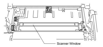
Fig. 5-22 Cleaning the Scanner Window
