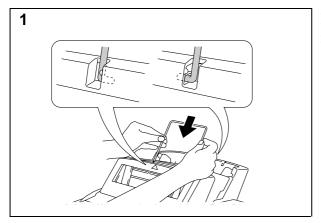
Install the paper support onto the front multi-purpose sheet feeder 1.
