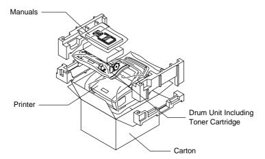
Fig. 5-28 Repacking the Printer
